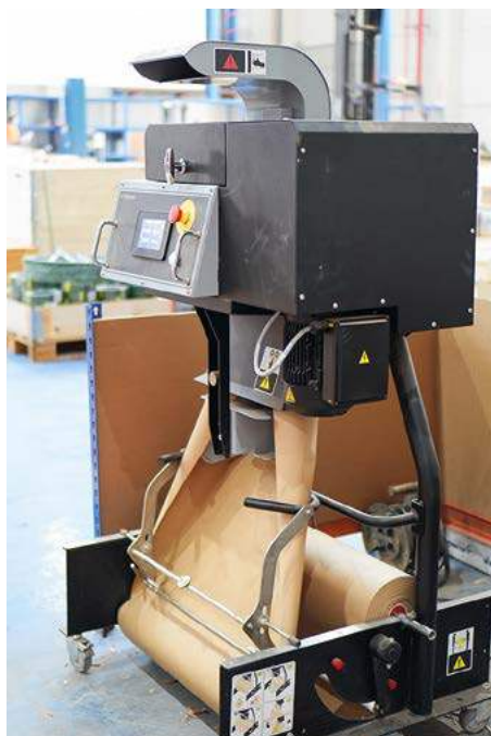
This paper cushioning system creates custom-length corrugated pads from 100% recycled paper.
