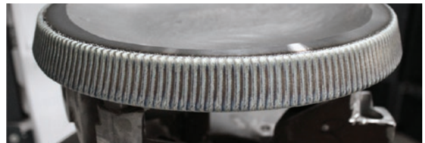
Laser cladding prior to machining
