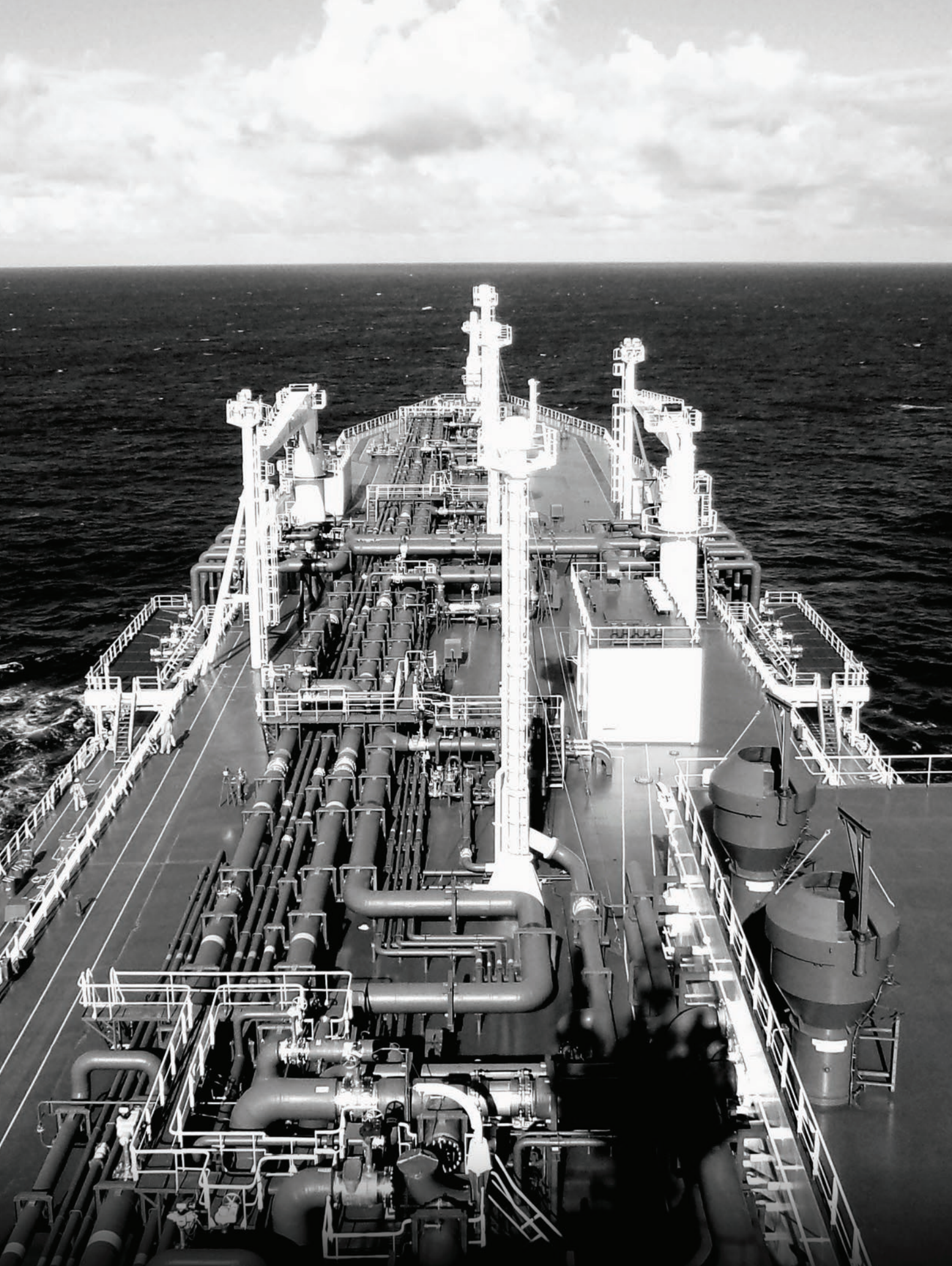
Top side pipelines of an LNG tanker with Westad valves. GTT no.96 membrane design.
